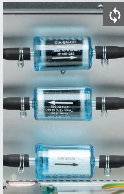
Gas conditioning with activated carbon and PTFE-filter
